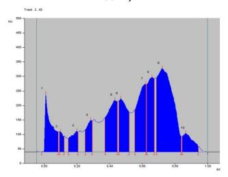
Fig. 3: HPTLC chromatogram area and peaks of the *Mimosa* pudica extract using Win CATS evaluation software (version 1.4.6.8121)
